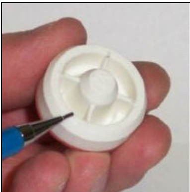
Examining the plunger seating surface
