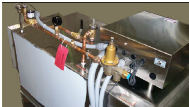
Incoming plumbing assembly for a Left to Right machine (note hole cover weldment in lower right corner)
